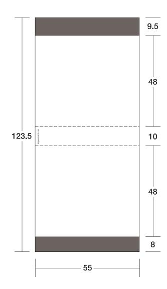
Bleed all 4 edges of background color 2mm to allow for folding and cutting in final production.
